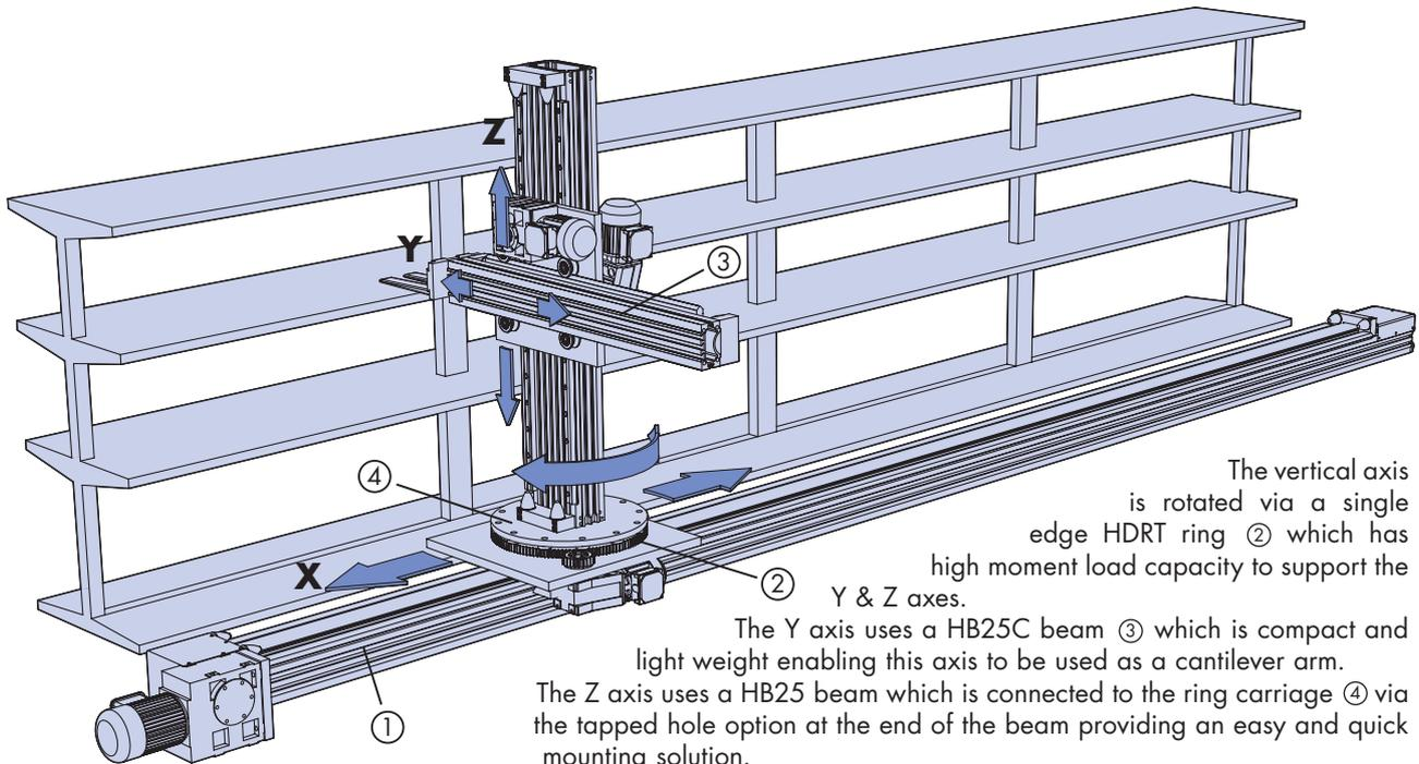
The vertical axis is rotated via a single edge HDRT ring ② which has high moment load capacity to support the Y & Z axes.
