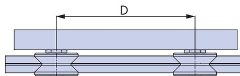
$$\text{Load Factor } L_F = \frac{L_1}{L_{1(max)}} + \frac{L_2}{L_{2(max)}} + \frac{M_s}{M_{s(max)}} + \frac{M_v}{M_{v(max)}} + \frac{M}{M_{(max)}}$$
