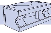
Cap wipers encapsulate the bearing when engaged with the slide and provide constant lubrication to the contact faces thereby greatly increasing load capacity and life. They prevent ingress of debris and improve safety and appearance. Lubrication is by means of sprung loaded oil impregnated felt wipers. The small series has a central cavity filled with grease which partially liquifies under operation and recharges the wipers.
