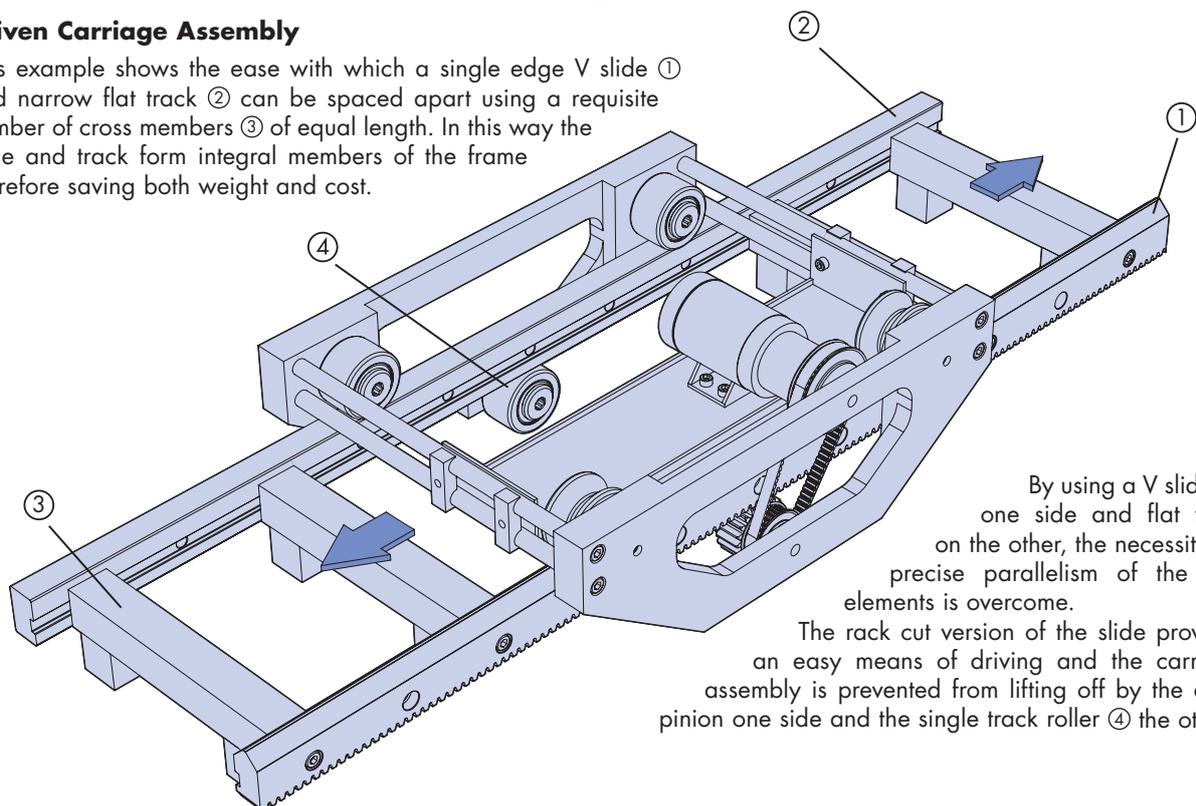
By using a V slide on one side and flat track on the other, the necessity for precise parallelism of the two elements is overcome.
