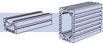
The design of Hepco construction beams enables slides and flat tracks to be factory assembled directly to the corner faces of the beam or, to be mounted at the many T-slot positions in conjunction with back plates and T-nuts 24&25. Very high stiffness allows the beams to be used as self supporting construction elements.
