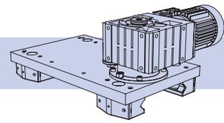
Hepco HDS2 rack driven carriages are available to suit the corner mounted options for construction beam assemblies or for other mounting arrangements with slides spaced the same distance apart 27. They are designed to engage with single edge V slides with integrated racks in precision, stainless steel and commercial grade options. They have all the benefits of the assembled carriages 26-27 with the addition of a high performance rack and pinion drive facility.
