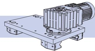
Rack driven carriages incorporate a strong drive flange assembly with micro adjustment facility to achieve correct mesh between pinion and rack 30. The standard design is for connection with Hepco supplied AC geared motors 31 this being the most economical means of achieving point to point linear motion. Speed and acceleration can also be controlled via an AC speed controller which Hepco also supplies.
