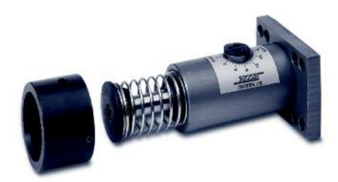
Hepco SH Shock Absorbers will match the speed and mass of the moving object and bring it to rest with no shock – the energy will simply be dissipated, mostly as heat. They also out-perform cylinder cushioning or dashpots, dissipating the energy at a uniform rate, thus enabling far faster stopping times to be achieved. The range offers adjustable and non-adjustable full threaded metric type shock absorbers together with fixed flange adjustable type up to 28mm bore size.
